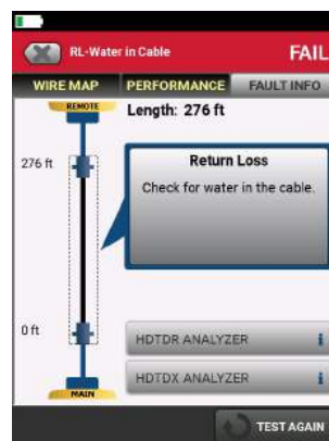
Cable that may contain water
