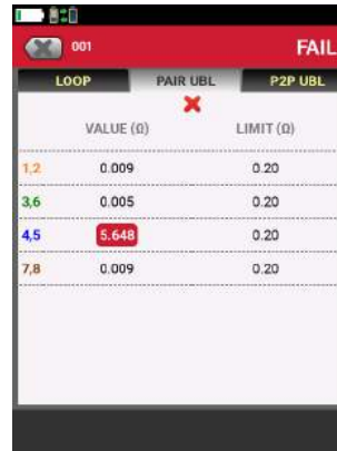
Excessive resistance which could cause an intermittent connection
